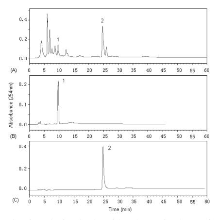
*Figure 3.* Results of HPLC analyses of the crude extract from the stems of *Edgeworthia chrysantha* lindl and its HSCCC fractions. Column: Shim-Pack CLC-ODS C<sub>18</sub> column (250 mm × 6 mm I.D.); mobile phase: acetonitrile–water in linear gradient elution (acetonitrile: 0-10 min, 35%; 10-30 min, 35–65%, 30-60 min, 65%); flow rate: 0.6 mL/min; UV detector: 254 nm (A) The original sample; (B) HSCCC fraction from Peak 1 (Fig. 2); (C) HSCCC fraction from Peak 2 (Fig. 2).
