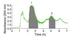
Fig. 2. Chromatogram of the essential oil of the rhizomes of *Curcuma wenyujin* by preparative HSCCC. Peak 1: germacrone; Peak 2: curdione. Solvent system: petroleum ether–ethanol–diethyl ether–water (5/4/0.5/1, v/v); stationary phase: lower aqueous phase; mobile phase: upper organic phase; flow-rate: 1.0 ml/min; revolution speed: 670 rpm; sample: 658 mg diluted in 18 ml mixture solution of lower phase and upper phase (1:1, v/v); retention of the stationary phase: 85%.
