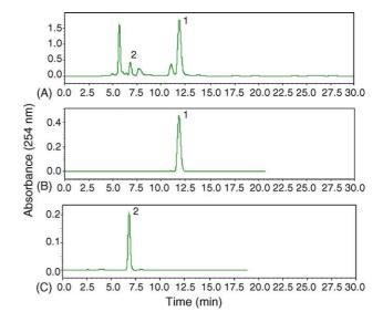
Fig. 3. The result of HPLC analyses of the essential oil and the partially purified sample from the essential oil. Column: Shim-Pack CLC-ODS  $C_{18}$  column (250 mm × 4.6 mm i.d.); mobile phase: methanol–water (85:15, v/v); flow-rate: 0.8 ml/min; (A) The essential oil; (B) HSCCC fraction from peak 1 (Fig. 2); (C) HSCCC fraction from peak 2 (Fig. 2).
